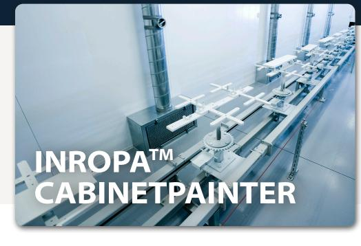
Inropa<sup>TM</sup> CabinetPainter automatically programs the robot by 3D-scanning the parts. Inropa<sup>TM</sup> CabinetPainter ensures high surface quality, reduces costs for personnel and paint material and increases production by ensuring a constant and optimized paint line flow.
