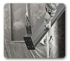
Inropa<sup>™</sup> SteelPainter makes painting easier and creates reliable results. the conveyor and sends them through the paint line. Inropa™ SteelPainter then scans the parts and programs the robots on the fly. This means that no human robot programming is necessary.
