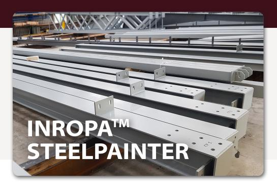
Inropa<sup>TM</sup> SteelPainter automatically programs the robot by 3D-scanning the parts. Inropa<sup>TM</sup> SteelPainter ensures high flexibility and surface quality and reduces costs for personnel and paint material. It increases production by ensuring a constant and smooth paint line flow.
