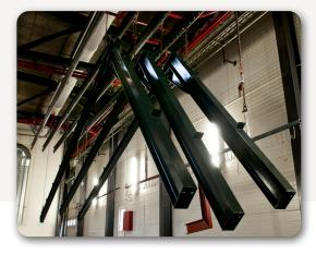
The operator mounts the parts on the conveyor, and the parts are then sent through the paint line and scanned in 3D. From these scans, the Automatic Programmer generates the robot programs automatically.
